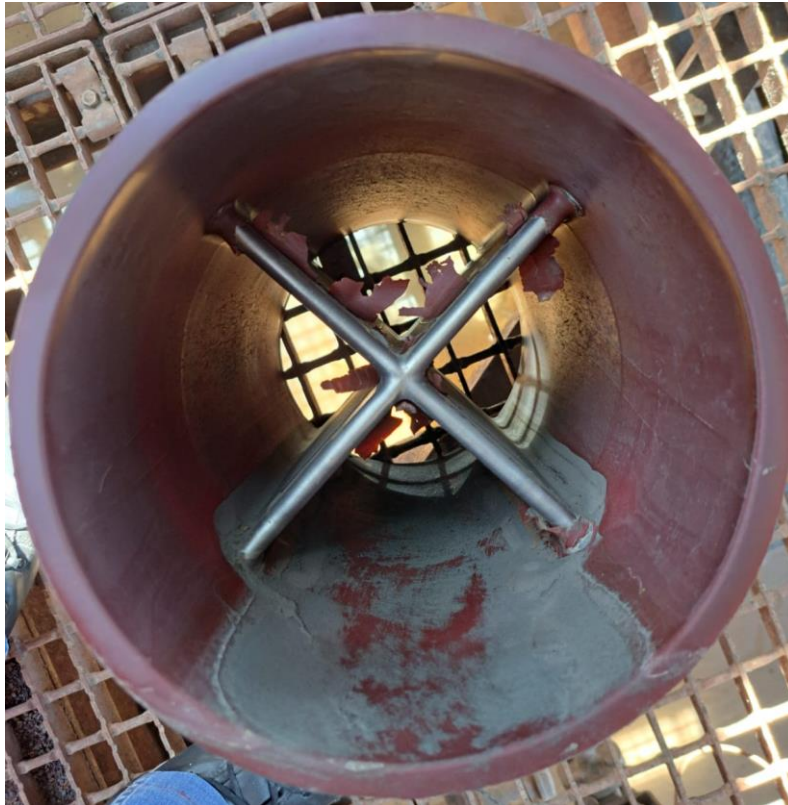
Figure 7 - Flow Corrector Wear
